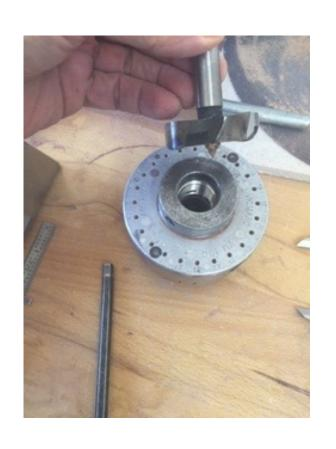
Drill the wood with the forstner to the depth of your chuck's insert This so the chuck will lay flat on the wood
