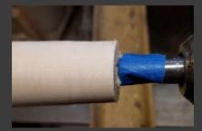
3. Physically measure and mark the depth of the inside hole.
