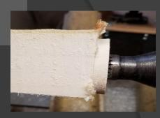
2. Drill the blank. I typically use a ½" drill, to a depth of 3".
