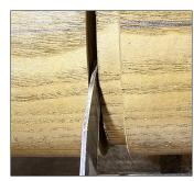
6. Cut your tenon to approximately 1<sup>1</sup>/<sub>2</sub> the width of the wider parting tool (roughly <sup>3</sup>/<sub>8</sub>" in this case). This gives you a deep tenon for a good friction/suction fit, and prevents the tool from binding in the cut, which can create dangerous catches (photo to the left). At the bottom of the tenon, part with a thin kerf parting tool, again, cutting about twice the width of the tool to prevent binding (Photo left, below).
