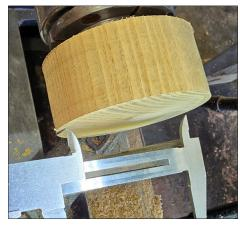
put the bottom half of the box in the chuck. 8. Flatten the face of the bottom half of the box. Remove as little wood as possible again, the more you remove from between the top and the bottom, the
