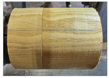
9. Align your pencil marks, or a grain feature, and fit the top to the base of the box (photo above). Do not hollow the base before rejoining the halves and turning the outside of the box. This ensures the base maintains the strength to support your friction fit while turning the outside of the box. Safe practice is to return the tailstock to support the entire piece until the last
