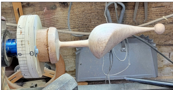
Jig centered, turn leg and base.
