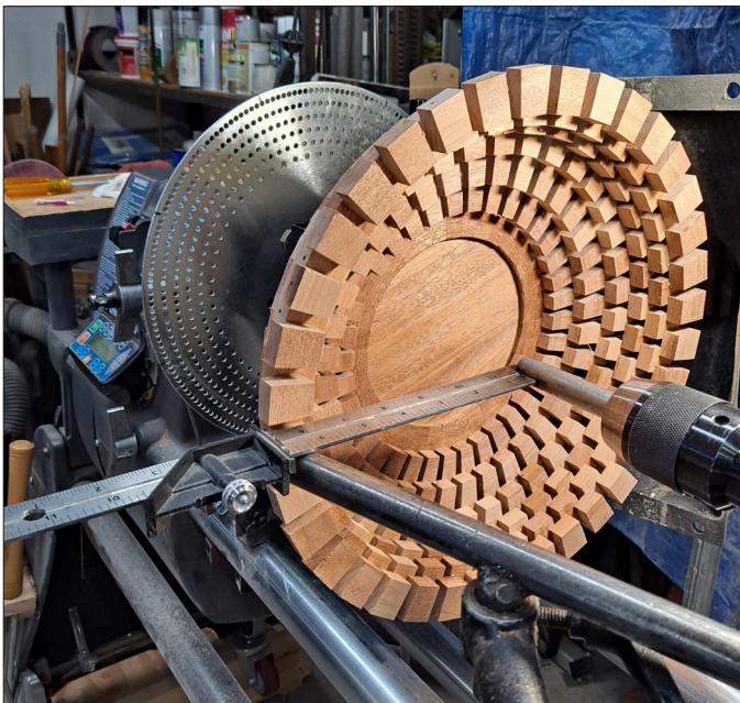
Select a new index hole and glue on the next piece until all segments are in place completing the ring.
