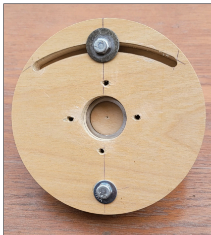
Washer added to prevent the screws that hold the turning blank from digging in to the wood on the back of the jig.
