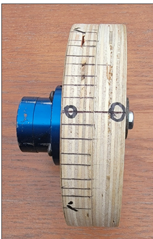
Washer added to prevent the screws that hold the turning blank from digging in to the wood on the back of the jig.
