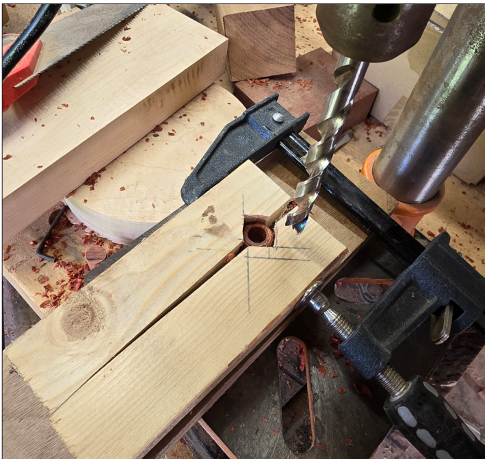
No specialized way to hold small, round pieces like beads for drilling? Editor Joaquin Juatai made this quick, easy jig to hold beads. Split a piece of waste wood down the center, cut corresponding 90-degree notches, and use a standard "F" style clamp to hold your work piece. Simple, quick, and safe.
