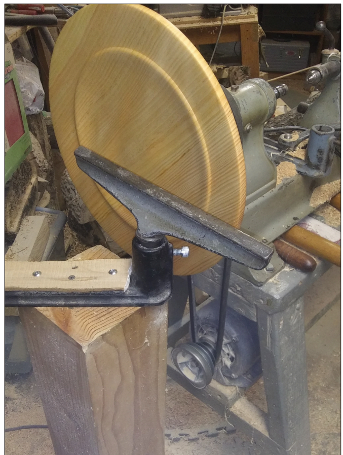
Jayson Cote Here you can see the banjo attached to the top of a 6x6" Douglas Fir pillar, giving Jayson a solid tool rest in order to turn this 14" White Pine platter.
