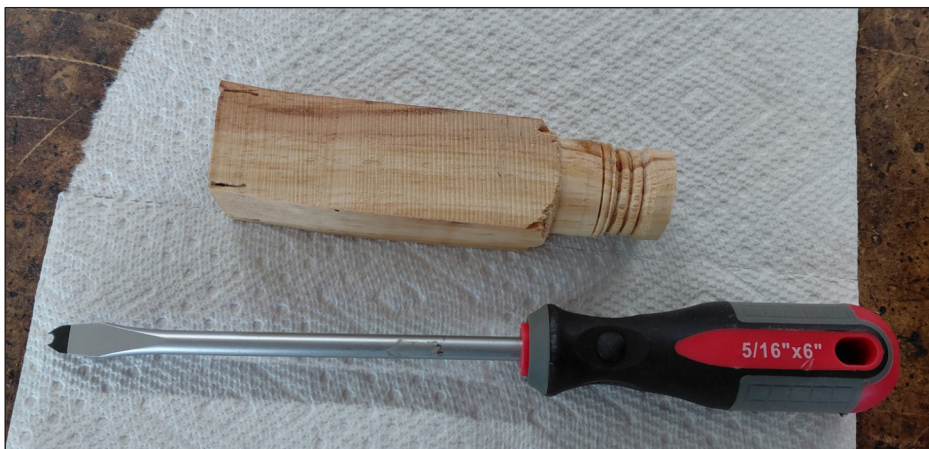
Bob Grinstead shared this 1/8" beading tool made using a Harbor Freight screwdriver ($3) shaped with a 3" cut off saw, also from Harbor Freight.
